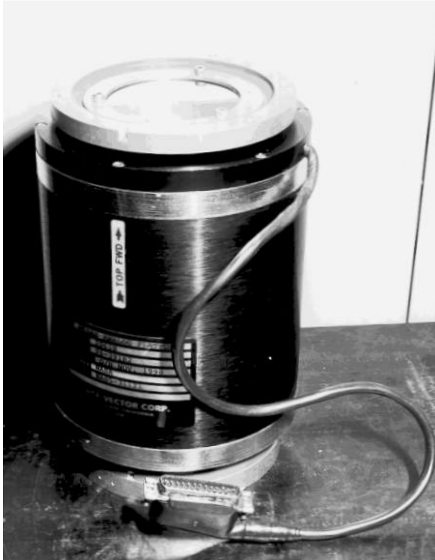
Figure 5-3. MIDAS Attitude Sensor
