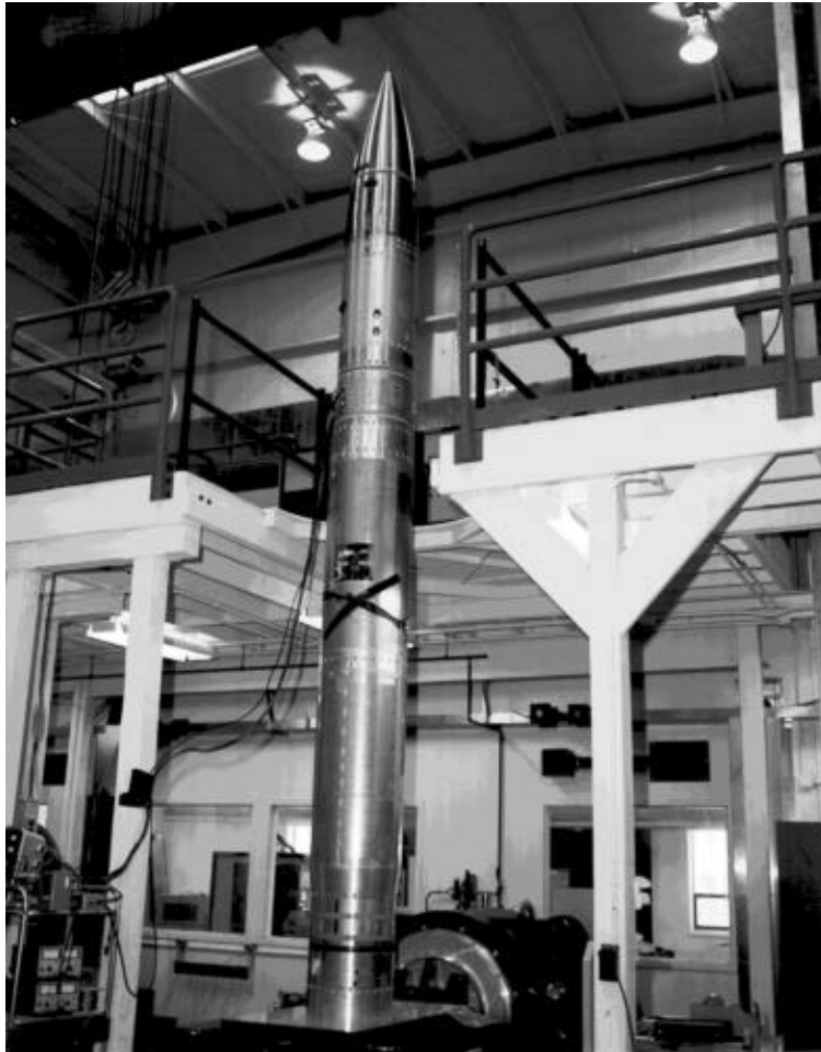
Figure 11-6. Astrophysics Payload (36.022) undergoing Lateral Vibration Testing
